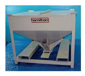
Portable Storage Bins were designed to replace gaylords in your bulk material handling system. You can buy material in bulk and use Portable Storage Bins to distribute the material throughout your plant. These 44" square, stackable bins can be filled using Surge Bins, Screw Conveyors or Hydraulic Dumpers. They can be discharged though the 4" bottom slide gate or the optional 4 way vacuum ports.
