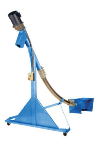
The Hamilton Granulator Unloader is designed to replace the catch box on many brands of granulator. These units will deliver up to 2000 pounds per hour of ground plastic to a Gaylord container or portable storage hopper. These durable, economical units relieve your operator from having to check the fullness of drawers and emptying them, saving both down time from over packed drawer and your operator's back.
